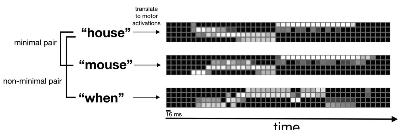
**Fig. 3.** Pattern discrimination task. Spoken words are converted to sequences of motor activations on the wristband. Three examples of 524 stimuli are shown.
