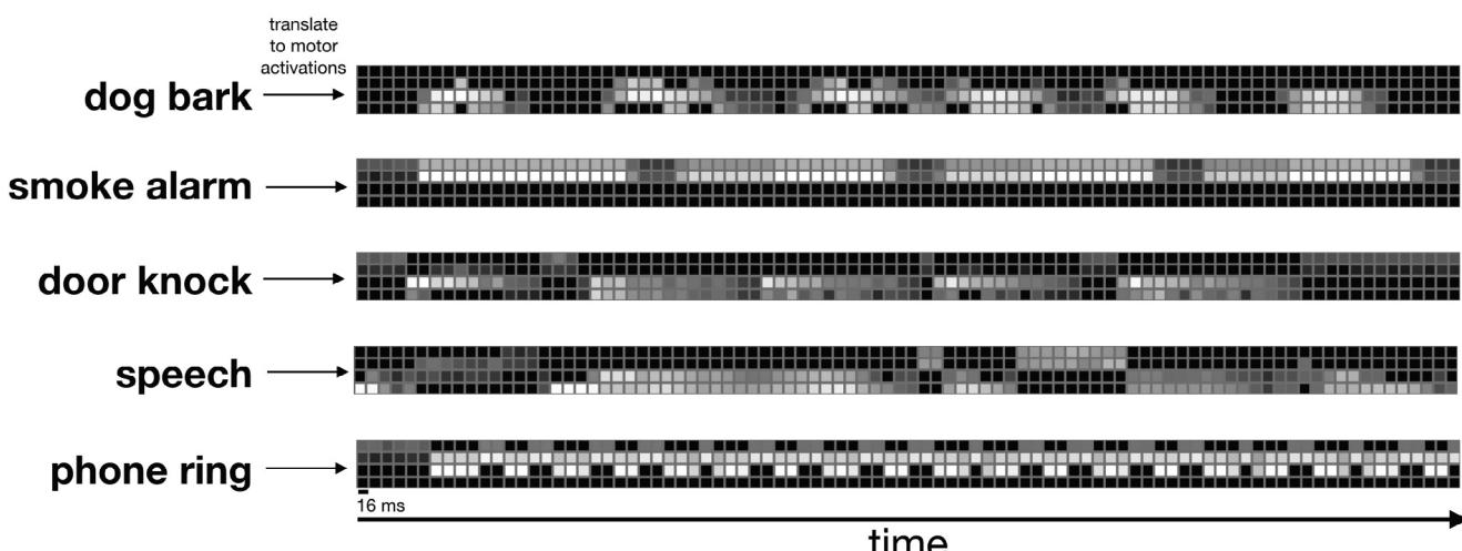
**Fig. 2.** Sound identification task. Sound files were algorithmically translated into patterns of motor activation. When two motors are active, an illusory position in between their locations is perceived. Five examples of 70 stimuli are shown.
